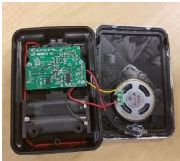
Appendix 1, Figure 4. Inside a wireless doorbell receiver. Soldered wires connect to ground (black) and positive charge (red).
